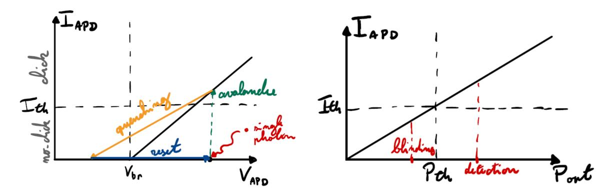
By shining continuous light in Bob's detector, Eve can make the avalanche photodiodes work in a linear regime.
