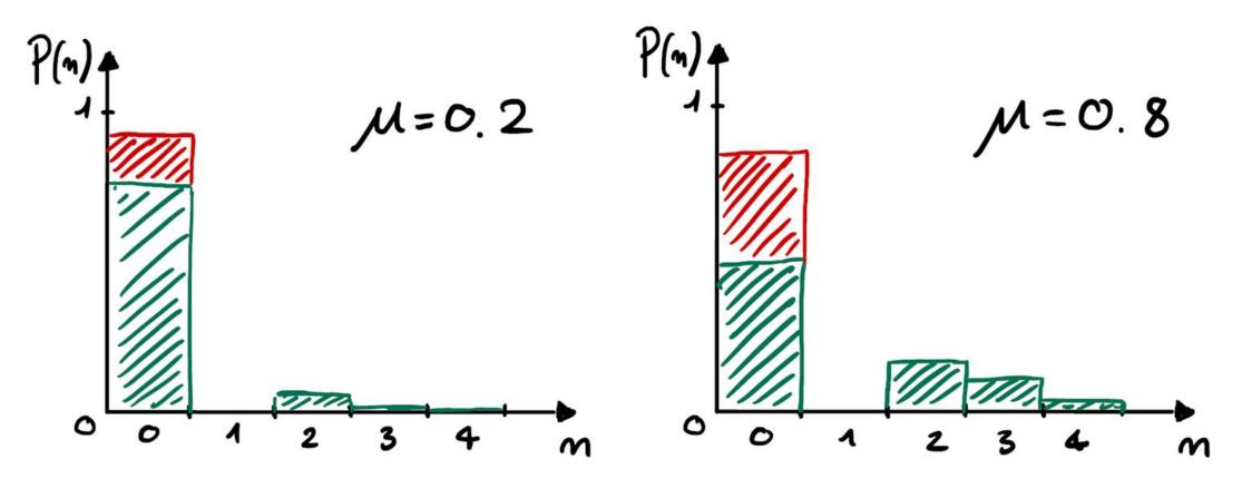
In this case a PNS attack changes the probability of detection with respect to the decoy intensity -> it can be spotted.
