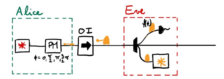
An easy countermeasure is using an optical isolator
