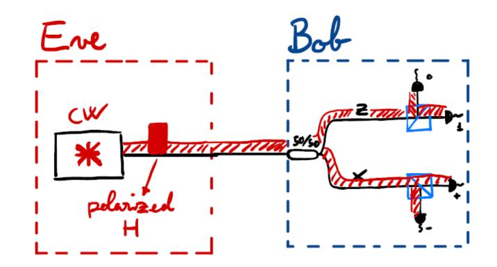
By adding power in a chosen polarization, Eve can induce a detection in the respective detector.
