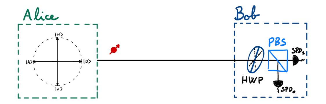
Used mostly in free space communication. In fiber requires an active tracking of the polarization.
