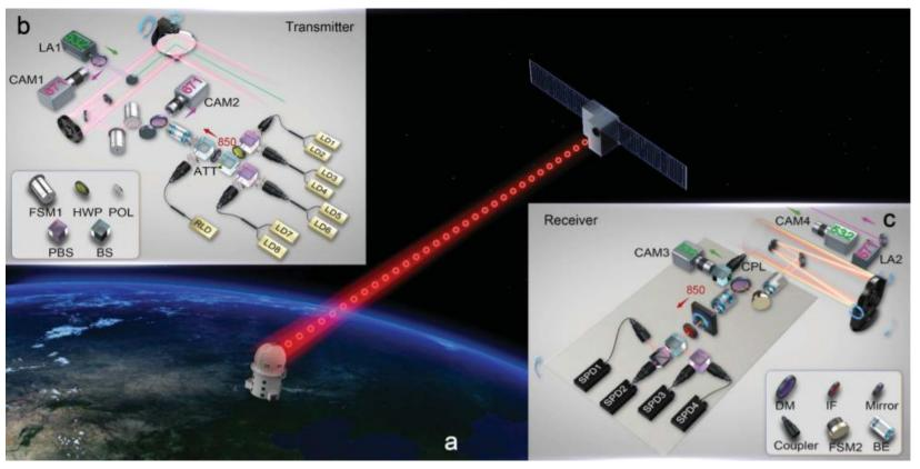
Decoy state BB84 protocol Polarization encoding.
