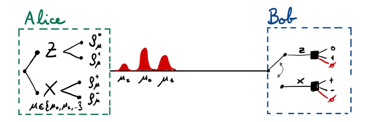
We can modulate the intensity of the phase-randomized coherent pulses
