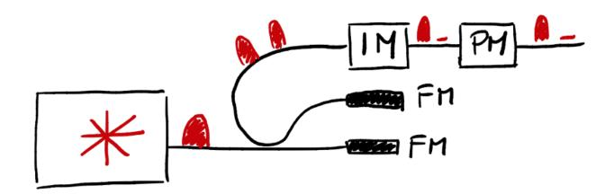
Michelson interferometer with Farady mirrors to avoid polarization dependence
