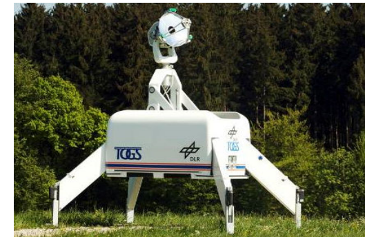
2013: First air-to-ground link Mach 0.7, 1.25 Gbps, d=60 km jointly with ViaLight, Contract by Airbus
